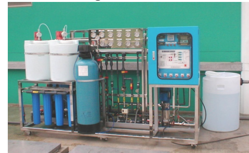
RO Pilot System (Capacity: ~1.5 m 3 /day)
