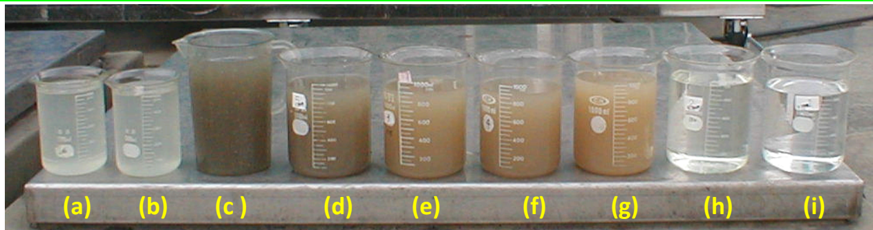
(a):raw wastewater, (b): PH adjustment, (c): anoxic tank, (d~f): aeration tank, (g): MBR membrane tank, (h): MBR membrane permeate, (i): RO permeate
