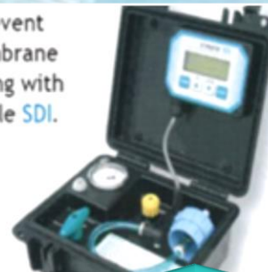
SDI (efficiency test for Pre-filter)
